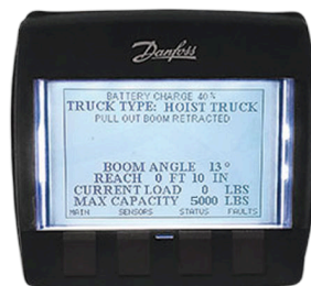
Rated Load Limiter Automatically detects attachment and adjusts loading parameters.
