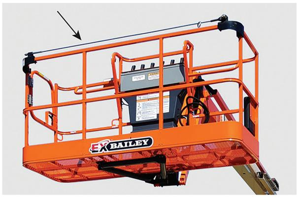
A Bolt-On Fall Arrest System can be bolted to existing JLG platforms in the field.
