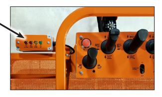
**Competitors Design:** Battery Condition Indicator located at ground only. Away from operator. What would happen if machine stopped in the middle of a painting operation?
