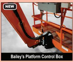
The competition still uses hydraulic joysticks requiring many hoses to route through cable tracks to the platform. Hydraulic joysticks have been replaced by electric over 20 years ago due to the maintenance and leakage nightmare. The competition has 27 hoses and 38 fittings at the platform. A high pressure hydraulic leak or blown hose could ruin a paint job!
