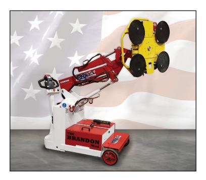
Model: Brandon Mini Hook Capacity: 1,000 lbs Glass Capacity: 700 lbs Power: 24 Volts Boom: Proportional Telescoping Boom Steering: Rear Wheel Drive: Rear Wheel Electric Motor Weight: 2,000 lbs Material Lifting: Optional 1000# Lift Hook Charger: On-board 110 Volts
